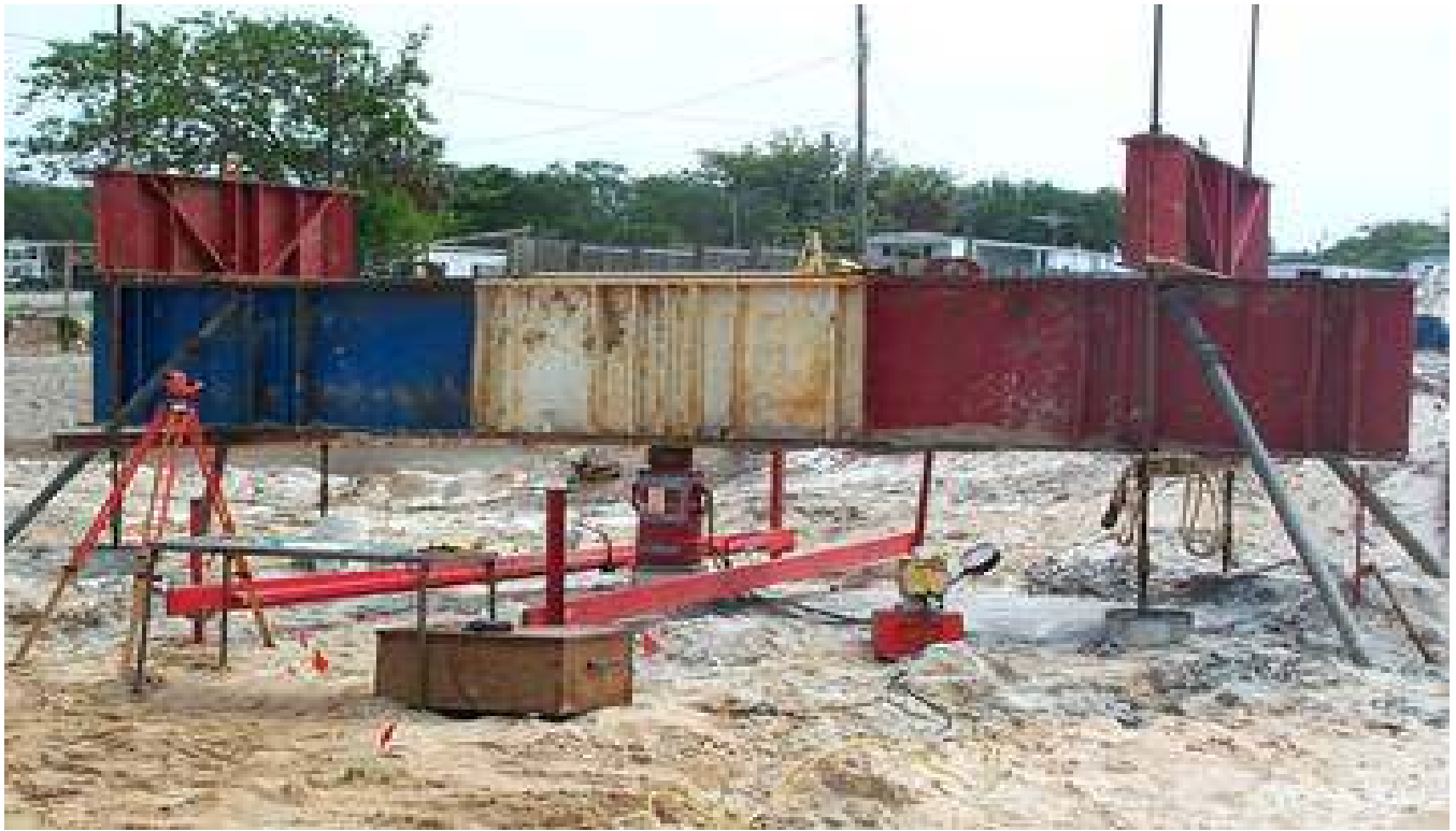
Figure 2- View of static load test on Pensacola Beach in Florida.
