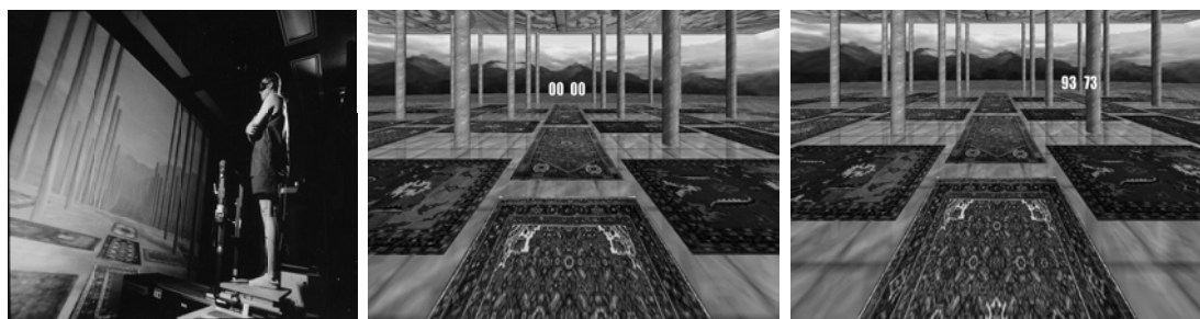
Figure 1. (Left) Subject wearing stereo shutter glasses stands on the posture platform in front of the back projection screen. The virtual image with a projection of the stationary no-calculation task (centre) and the randomly moving calculation task (right).
