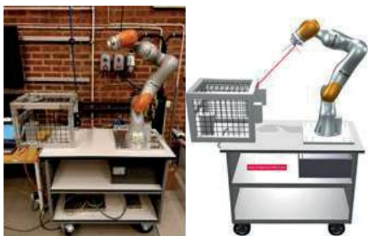
Fig. 8. Physical robot (left) and its virtual representation (right)
