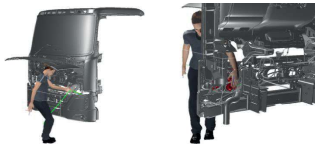
Fig.6. Truck headlight bulb replacement simulation. The path in green connects the initial position and the goal position. Before approaching the truck, the manikin was in a standing pose with feet together and arms by the sides. Truck CAD model courtesy of AB Volvo.
