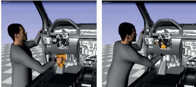
Fig. 7. Simulation of assembling the Central Electronic Module (CEM). Car CAD model courtesy of Volvo Cars.
