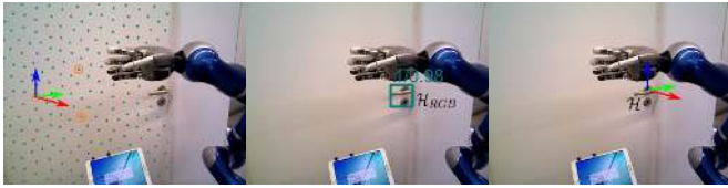
(a) Plane estimation. (b) Box detector. (c) Handle position. Fig. 6: Pipeline for the door handle position estimation.
