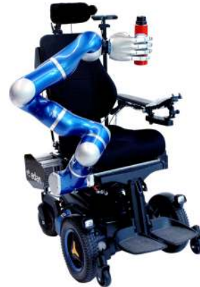
Fig. 1: The assistive robotic system EDAN (EMG-controlled daily assistant).
