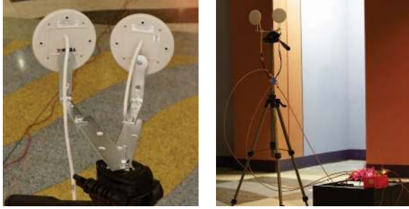
(a) 5dBi directional patch antennas at the prototype full-duplex base station (b) Front view prototype full-duplex base station with directional antennas mounted
