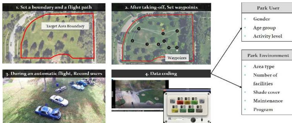
Fig. 2: Park-user data collection process using UAVs
