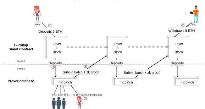
Figure 4. A transaction's life cycle on a zk-rollup. Tx batch refers to a batch of transactions.
