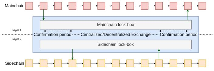
Figure 1. Illustration of a two-way-peg mechanism.
