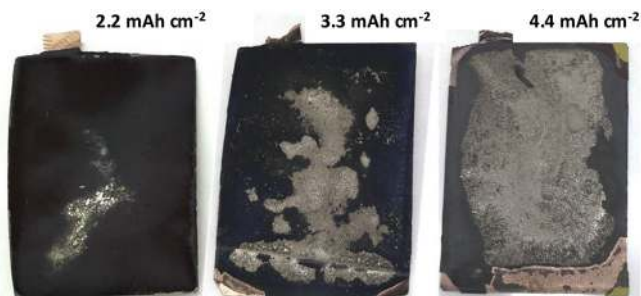
Fig. 2. Evidence of increasing lithium deposition (metallic gray) on graphite electrodes as a function of capacity loading. From Ref. [21].
