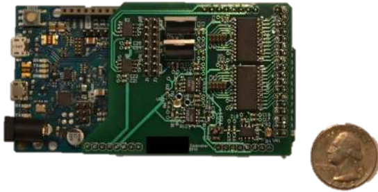
Figure 11—MoVR mirror’s controller board: The figure shows our custom-designed controller board for configuring the beam alignment and the amplifier gain in real time.
