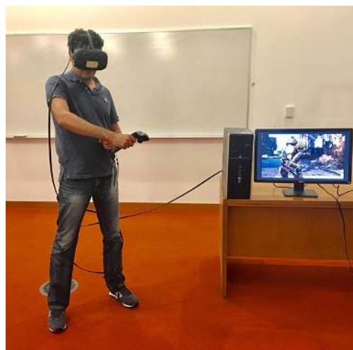
Figure 1—Virtual Reality experience: The figure shows the headset's cable not only limits the player's mobility but also creates a tripping hazard.
