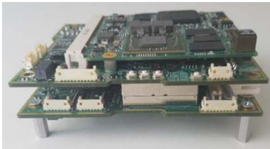
Fig. 4 Photograph of SpaceCloud™ iX5 CORE and EXTENSION module stacked with compute module attached at the top
