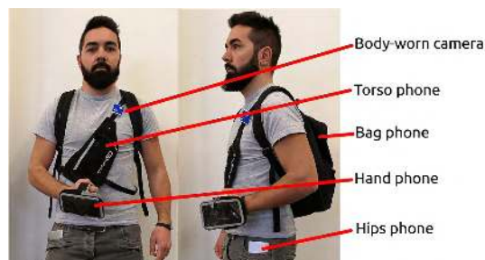
FIGURE 2. A participant wearing the four smartphones and a camera during data collection.
