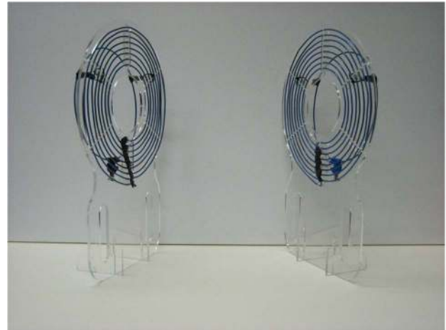
Fig. 3. Image of the two high-Q MCRs used for wireless power transfer. These coils will be used as an experimental reference throughout this work and are referred to in the text as the “blue coils,” since the insulation used to coat the wires is blue. The outer radius of the coils is 14 cm, and a detailed summary of their properties can be found in the Appendix.
