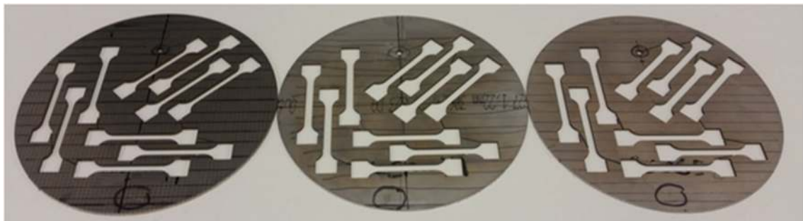
Fig. 5 Tensile Samples cut from blanks showing orientation
