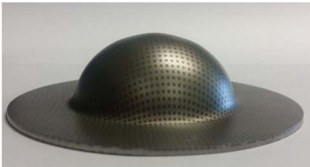
Fig. 15 6.35 mm edged C263 with a slightly crushed top
