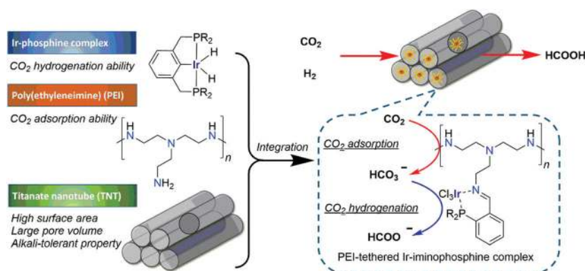
Fig. 22 Schematic illustration of Ir-PN-PEI@TNT(Na + ) 106 mediated CO 2 hydrogenation. 139
