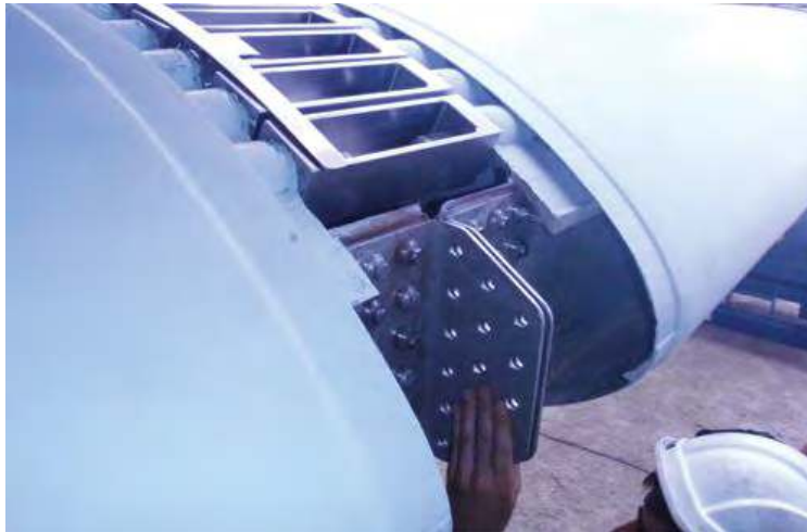
Figure 5-9. Jointed wind turbine rotor blade
