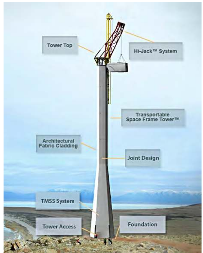
Figure 5-6. Conceptual diagram of the space frame tower system™
