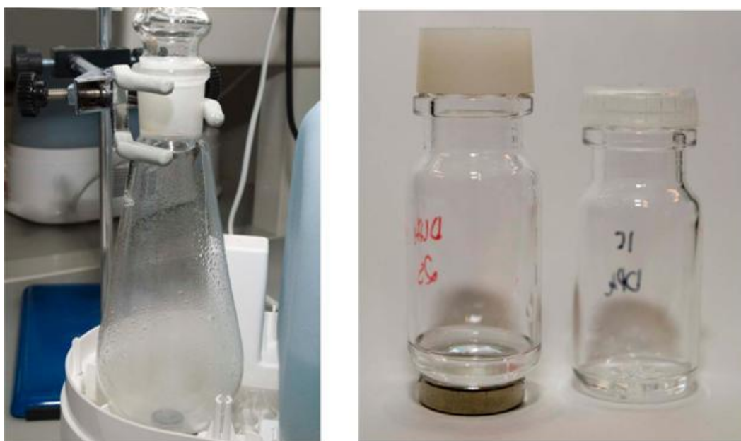
Figure 1. Water-air induced crystallization setups. (Left) Aerosol experimental setup. Here the flask has a magnet within the crystal vessel with the South pole facing upwards. (Right) Steady crystallization experimental setup, one vessel with magnetic field and one without.
