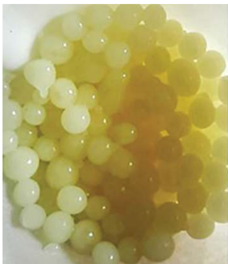
FIGURE 3 - Photograph of the spherical calcium alginate/salep beads of flaxseed oil extract.
