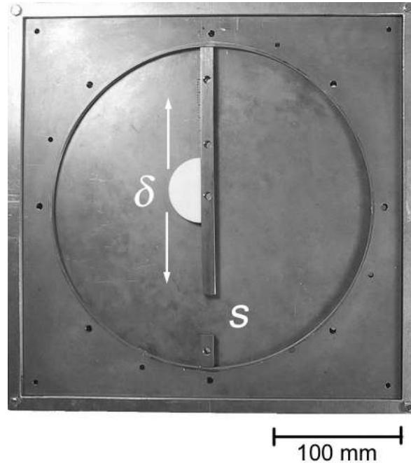
FIG. 2: A photograph of the opened microwave billiard employed for the observation of EPs. A circular copper cavity is divided into two semi-circular parts. The two parts are variably coupled by a slit of width  $s$ . One of the semi-circular cavities can be perturbed by adjusting the position  $\delta$  of a teflon stub inside the resonator.
