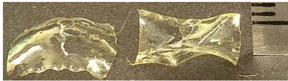
FIG. 3: (Color online) Positive (left) and negative (right) Gaussian curvature in 15\ \mu\text{m} thick glassy liquid crystal network at 175^\circ\text{C} .
