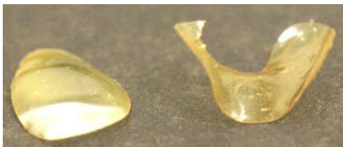
FIG. 5: (Color online) Side by side comparison of positive (left) and negative (right) Gaussian curvature realization in actuated elastomeric films.
