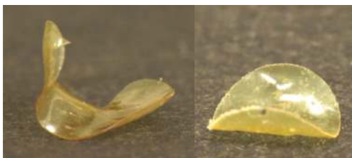
FIG. 6: (Color online) Comparison of shape selection of discs in the negative Gaussian curvature case depending on the size of the domain. For smaller radii ( 3.7\ \text{mm} initial diameter) a saddle shape is formed as expected (right). When the radius of the disc is sufficiently large ( 7.1\ \text{mm} initial diameter), considerably more complex surfaces with wavy edges are formed (left).
