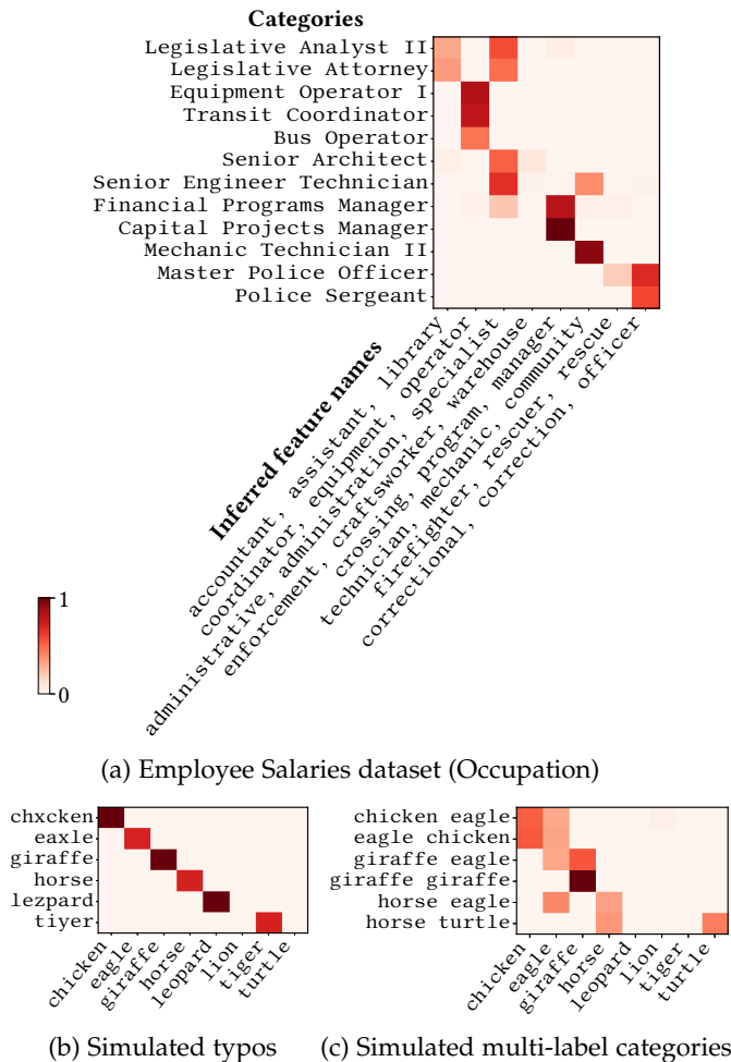
Fig. 4: Gamma-Poisson factorization gives positive and sparse representations that are easily interpretable. Examples of encoding vectors ( d=8 ) for a real dataset (a) and for simulated data (b and c) obtained with a Gamma-Poisson factorization. The x -axis shows the activations for each dimension with their respective inferred feature names. Figure 14 in the Appendix shows that other encoders fail to give such an easily-understandable picture.
