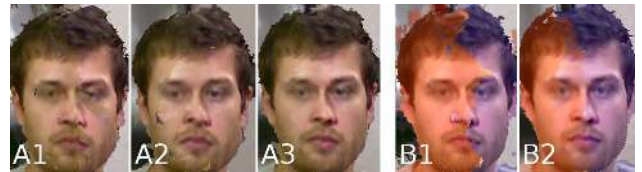
Figure 9: Data merger results. A1: No merger applied, meshes drawn on top of each other. A2: Merger with simple average. A3: Merger with quality weighting. B1: Color coded camera contributions with no merger. B2: Camera contributions with quality-weighted merger.
