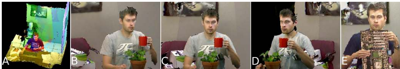
Figure 1: Left to right: A) Camera coverage with five color-coded camera contributions. B-D) Three views of a live capture session. E) A 3D virtual object (circuit board) is incorporated into a live 3D capture session and appropriately occludes real objects.
