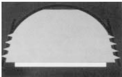
Figure 15 Hemispherical shell with conical threads.
