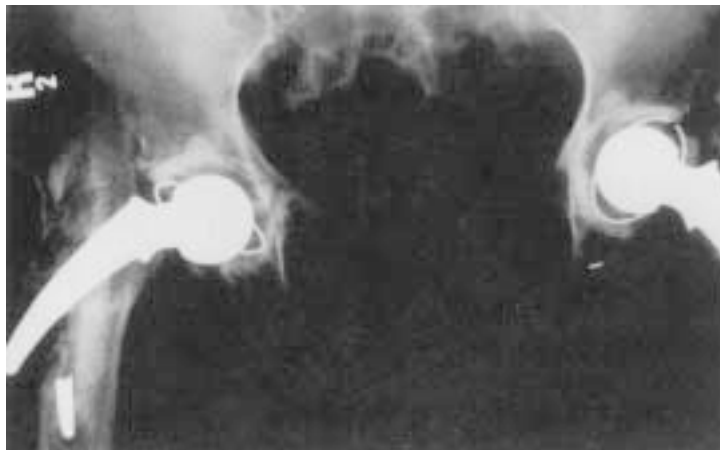
Figure 51 Fractured cemented stem.
