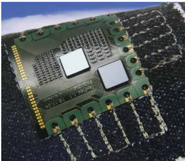
Figure 5-2 Embroidered flexible PWB on textile substrate
