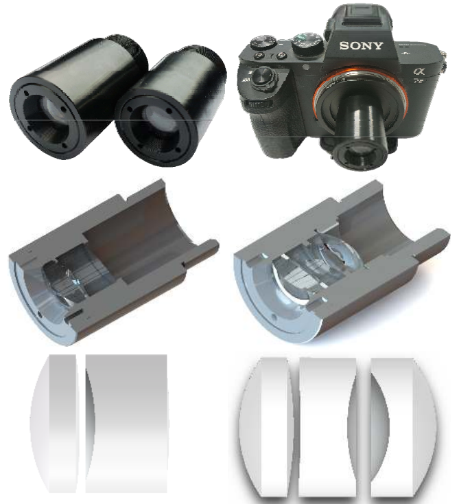
Fig. 4. Prototypes and the rendered section views of our designed lenses. The top left shows our fabricated lens for LFOV (left) and EDOF (right) imaging, and the corresponding structures are shown in the medium/bottom left and medium/bottom right, respectively. The top right shows the assembled prototype with the camera body.
