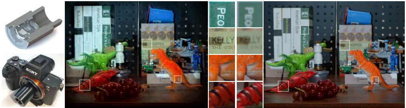
Fig. 1. An exemplary triplet design for extended depth-of-field imaging optimized by our end-to-end differentiable complex lens design framework. Top left: 3D model of the optimized triplet lens design ( 50\text{mm}/F4 ). Bottom left: prototype fabricated by single-point diamond turning. Middle: final image that is captured by our end-to-end designed lenses and processed by our algorithm. Right: the same scene captured by a Sony 28 – 70mm zoom lens at 50\text{mm}/F4.5 . The objects are placed in the range from around 0.8\text{m} to 1.8\text{m} from the lenses. Our prototype succeeds in obtaining the all-in-focus image, while the conventional lens shows a narrow depth of field.
