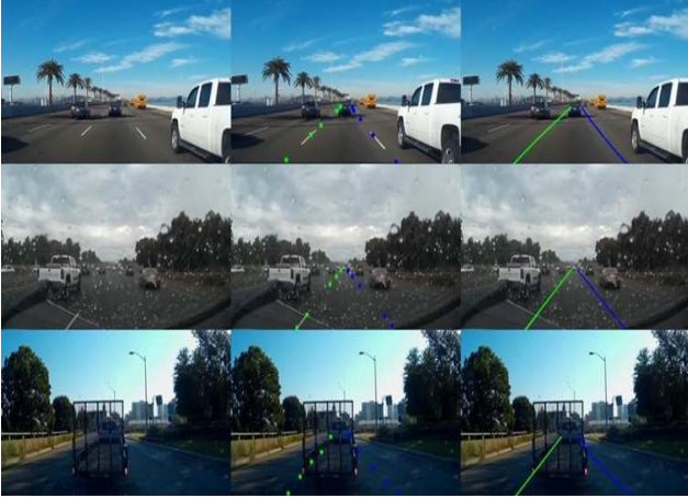
Figure 2. Semi-automatic interface to annotate left and right ego lanes. Original image (left). Annotation of lane points (center). Fitted curves (right).
