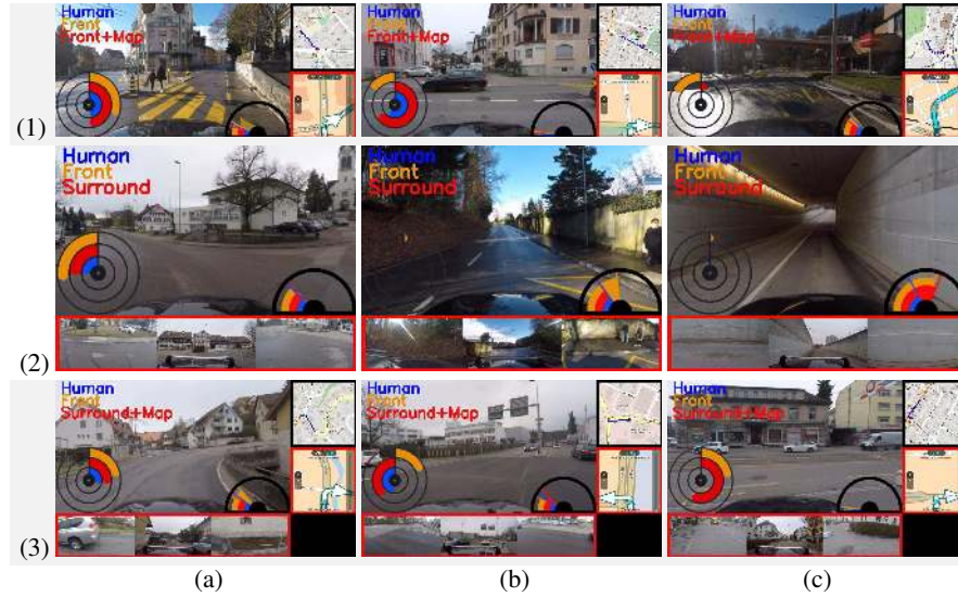
Fig. 3: Qualitative results for future driving action prediction, to compare three cases to the front camera-only-model: (1) learning with TomTom route planner, (2) learning with surround-view cameras (3) learning with TomTom route planner and surround-view cameras. TomTom route planner and surround-view images shown in red box, while OSM route planner in black box. Better seen on screen.
