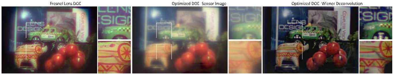
Fig. 6. Experimental results for achromatic extended depth of field imaging with DOEs. Left: an image captured through a Fresnel lens. Center, right: an image captured through a diffractive optical element (DOE) optimized with the proposed framework without (center) and with (right) Wiener deconvolution as a post-processing step. Over the scene depth range of 0.5 m to 2 m, the Fresnel lens displays significant out-of-focus blur at the extremes of the depth range and further suffers from significant chromatic aberrations. In contrast, the proposed optical element succeeds in focusing a wide range of depths for all three color channels, leading to an all-in-focus scene with little chromatic aberrations.
