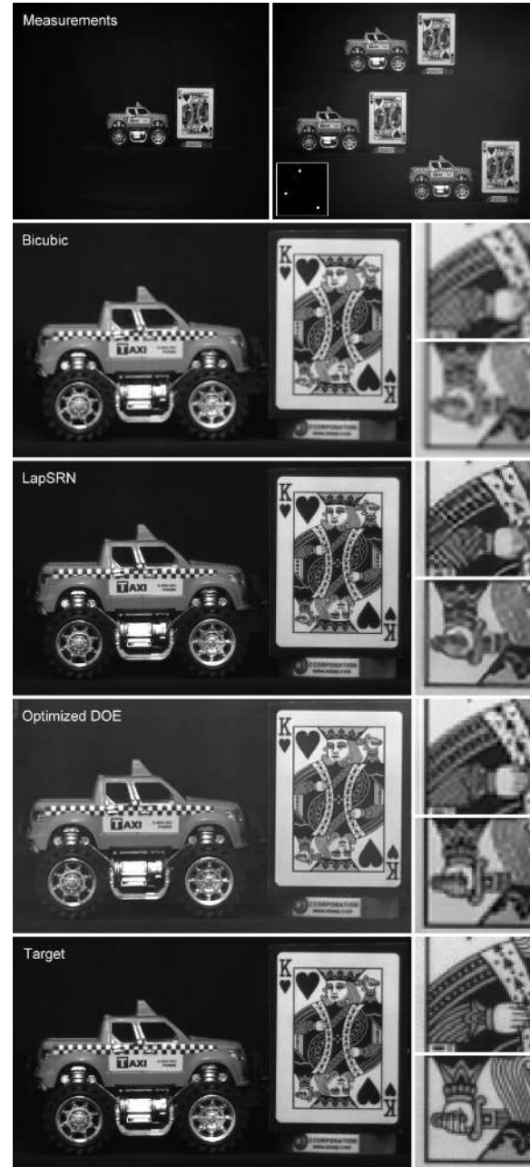
Fig. 9. Experimental result for 2 \times super-resolution. We capture an image with a conventional 35.5 mm lens (top left) and with the fabricated diffractive optical element (DOE) obtained with the proposed end-to-end optimization framework (top right, with PSF inset, blurred to increase peak radius for better visibility. Three peaks multiplexing the image are clearly visible.). As expected, the image recorded with the DOE creates multiple aliased copies of the scene. Bicubic upsampling of the scene (row 2) does not restore the fine details observed in the target image (row 5). Applying Lai et al.'s [2017] method (row 3) or other single-image super-resolution methods allows for high-frequency details to be hallucinated but these may be incorrect (i.e., hand, sword, ornaments). The proposed lens and reconstruction restores some of the true image detail better, even with the limited optical quality offered by our custom DOEs.
