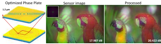
Fig. 4. Optimizing a simple optical element. We optimize a lens to focus an image at a distance of z = 25 mm without image reconstruction for a wavelength of \lambda = 550 nm. As expected, the optimized height profile (left) converges to a structure that looks similar to a Fresnel lens. As seen in the point spread function (PSF, center inset), the element is capable of focusing the green channel but residual blur remains in the other color channels because a single optical element cannot be achromatic. After deconvolving each color channel with their respective PSF, we obtain the result shown (right).
