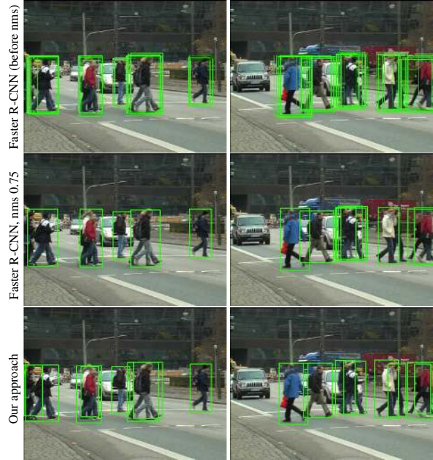
Figure 5: Example detection results on the TUD-Crossing dataset. Middle and bottom rows visualize output of Faster R-CNN and our detectors at the operating point with 90% precision. Top row shows output of Faster R-CNN before application of non-maximum suppression.
