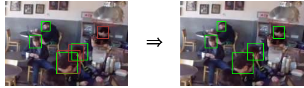
Figure 4: Example of stitching in a new region’s predictions (red) with accepted predictions (green).
