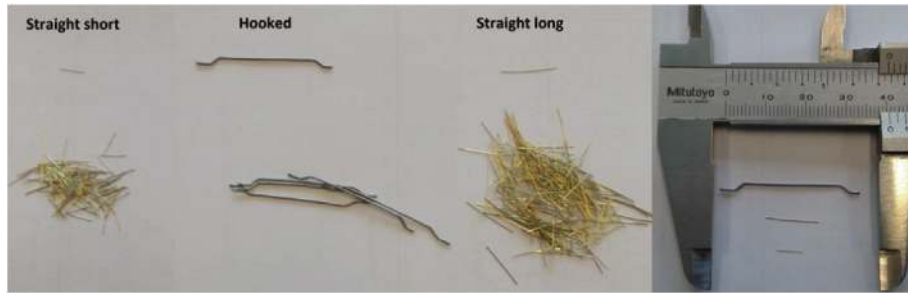
Fig. 2. Steel fibres used in this study.
