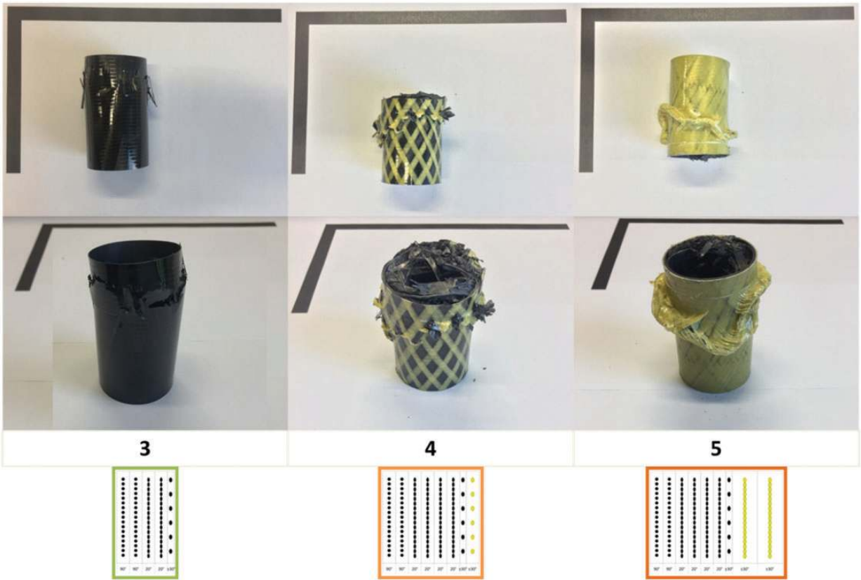
Figure 26. Pictures of CFRP tube specimens 3, 4, and 5 which underwent catastrophic failure for inner-crushing configuration (b).
