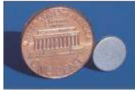
THERMOLIFE: 5200 BiTe thermocouples on kapton tape 123 \mu W @ \Delta T = 5K (42.5 \mu A at 2.9V)
