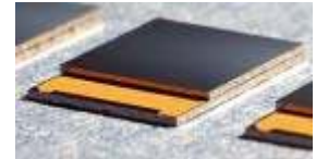
MICROPELT: BiTe thermocouples. 2.8mW @ \Delta T = 10K , (2.3V open circuit voltage)
