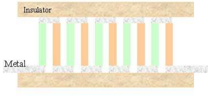
Figure 13: Schematic of thermoelectric converter (thermoelectric module).
