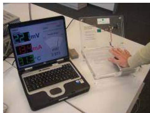
Figure 33: Picture of the Fraunhofer thermoelectric generator featuring a low voltage start-up circuit for [151]
