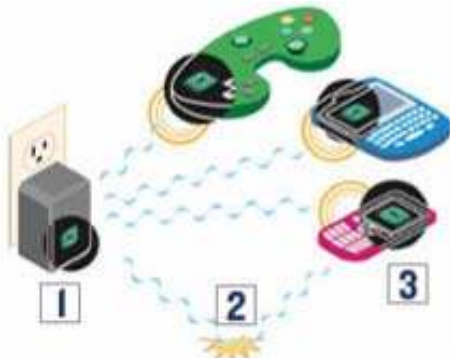
Figure 20: Solution by Powercast [30]: an RF transmitter (1) is plugged into a wall socket, it radiates radio waves (2) to tiny receivers integrated into devices (3).
