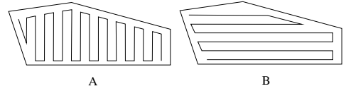
Fig. 10. The number of turns in path A is higher than in path B.
