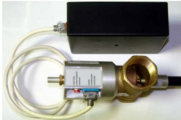
Fig. 11. Physical implementation of the wireless actuator: valve and transceiver with power supply in the housing
