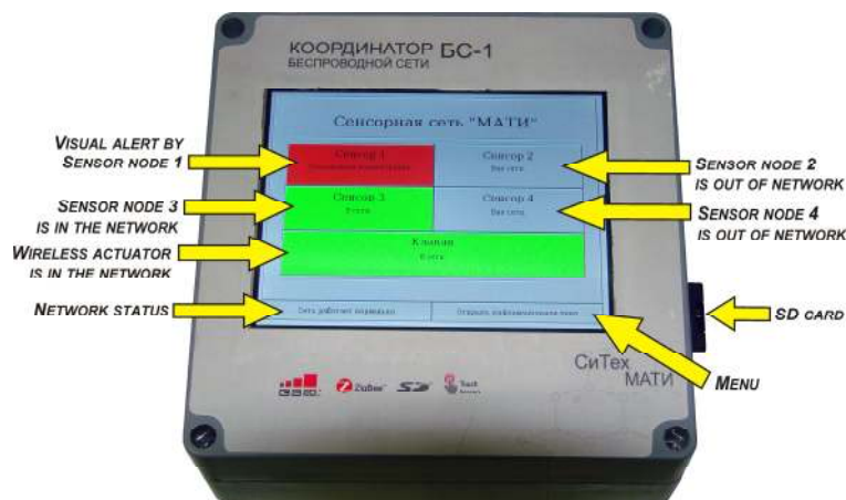
Fig. 10. The photograph of network coordinator where the highlighted sections on the display show the status of the WSN, the sensor nodes, and the wireless actuator(s)
