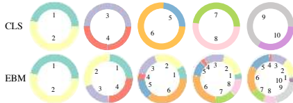
Figure 3: Predicted label distribution after learning each task on the split MNIST dataset. CLS only predicts classes from the current task while EBMs can predict classes for all seen classes.
