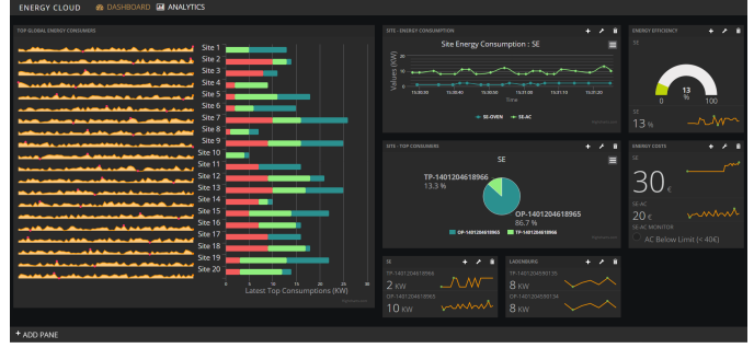
Fig. 3. Monitoring dashboard has a global overview of the energy consumption and the top consumers per site, and other individual measurements.
