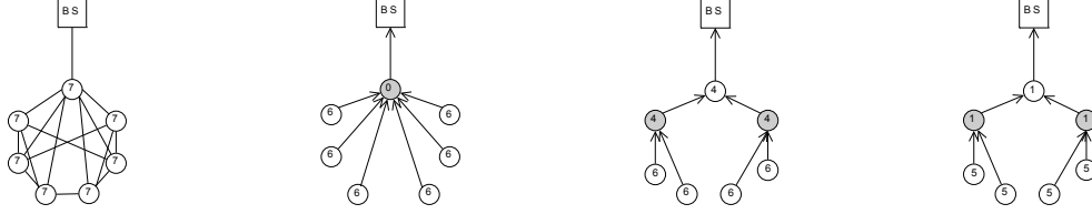
Fig. 1. Energy constraint clustering example: 1(a) Original Network 1(b) Without constraints after one round 1(c) With constraints after one round, 1(d) With constraints after two rounds
