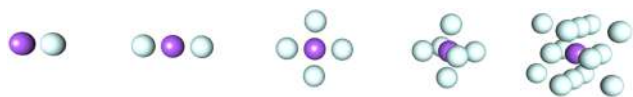
FIG. 6. Structures of the \text{NeHe}_N clusters, where N = 1, 2 (linear), 4 (square), 6 (octahedron), 14 (face-centered cubic). The distances between the center neon and the first layer of helium atoms are 3.43 Å, which comes from a ground state geometry optimization of the Ne–He dimer at the MP2/6-311(2+)G level.
