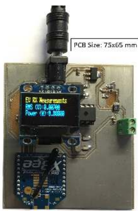
Fig. 7: RX PCB- interface between MRC-WPT circuitry and EV load
