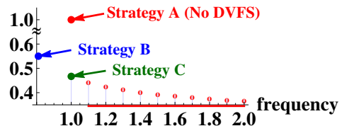
Figure 1: Normalized LO mode energy against the frequency of \tau_1 's extra workload, with the system energy consumption calculated in 48 ms, \alpha in (1) set to 2.5, f_{\min} set to 0.2, and the energy for Strategy A normalized to 1
