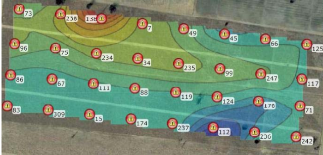
Fig. 4. Sensor arrangement in Belmont, The sink node is neighbor to node 96,86 and 83.
