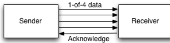
Fig. 1. Asynchronous pipelines: sender-receiver handshake protocol.
