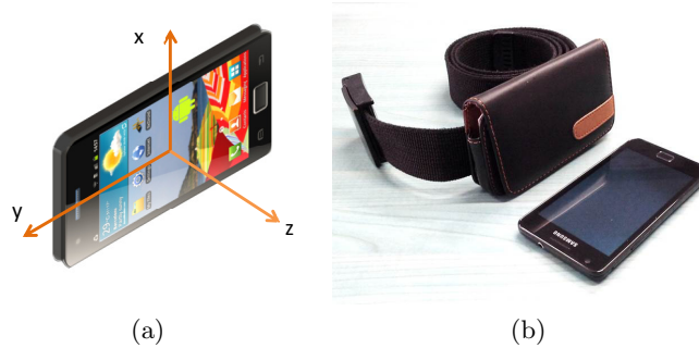
Figure 1: Samsung Galaxy S2 Smartphone. (a) arrows show the axis orientation of the accelerometer. (b) the smartphone case and belt used for the experiments
