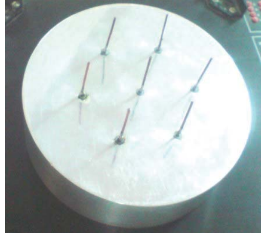
Fig. 4. Designed seven element parasitic switched array antenna.
