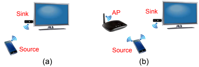
Figure 1: Network topologies for WiFi Display: (a) P2P topology for source’s local content streaming; (b) Two-hop topology for tethered streaming.
