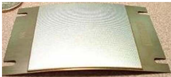
Figure 7. Dome-shaped piezo actuator (FACE International, http://www.faceinternational.com ).
