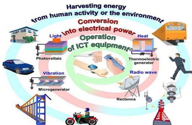
Figure 1. Energy harvesting and associative technologies, including vibrational microgenerator, solar Photo voltaic cell, thermoelectric, and rectenna, with potential applications in Information and Communication Technology equipment and assistive devices (adapted from Fujitsu Laboratories Ltd., http://www.fujitsu.com/ ).
