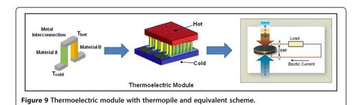
where  $S_A$  and  $S_B$  represent the Seebeck coefficients of the two materials. Thus, an electrical proportional current flows through the electrical load, which is connected in series with the thermo-electric generator.
