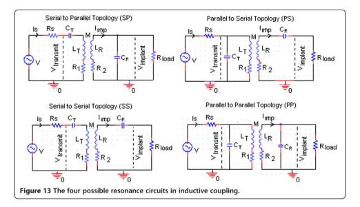
resistance of the power amplifier, whereas  $R_2$  is the effective series resistance of  $L_R$  as given by (Liu *et al.* 2005) [66] and (Harrison, 2007) [67]. The capacitors  $C_T$  and  $C_R$  are used to create a resonance on both sides of the link. The resonance frequency ( $\omega_o$ ) for an LC tank for both sides can be calculated as given in (7).
