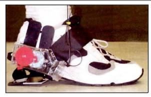
Figure 4 Magnetic generator adapted in a shoe.
