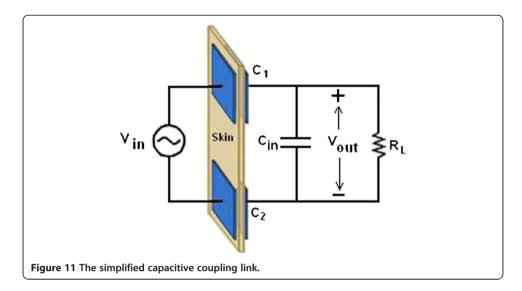
Referring to Figure 11, we analyzed the voltage transfer rate as follows:  $V_{in}$  is the input voltage,  $C_1$  and  $C_2$  are the capacitances between the implanted and external plates,  $C_{in}$  is the equivalent input capacitance of the implanted circuits, and  $R_L$  is the equivalent "ac" resistance of the loading network. The equivalent capacitors Ceq is given in
