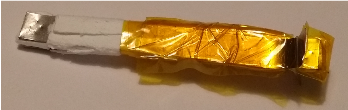
Figure 3.12: Assembled 55 mm harvester from Ni and Mo foil spot welded together, insulated with polyimide tape on the cold side and glass fiber on the hot side.
