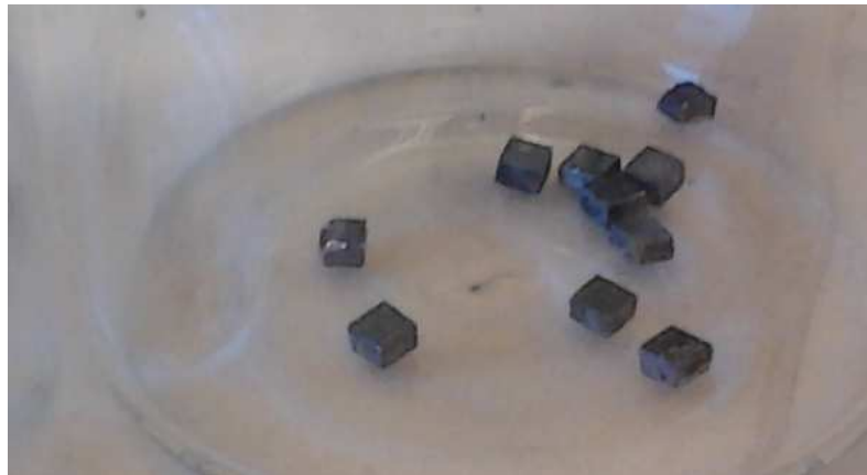
Figure 3.6: The size ( 1.6 \text{ mm} \times 1.6 \text{ mm} \times 1 \text{ mm} ) of the thermoelectric legs in the harvester. The material in this picture is \text{Ba}_8\text{Ga}_{16}\text{Ge}_{30} .
