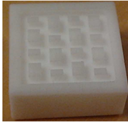
3.7.1 (b) PTFE mold with an area-ratio of 1:2.6.
