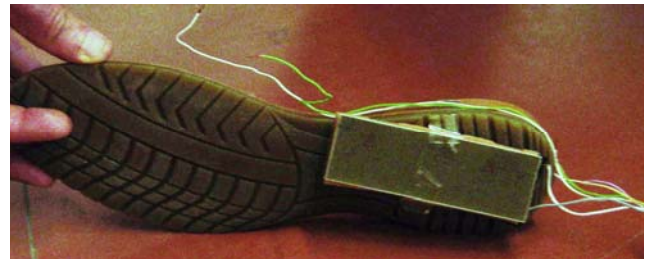
Fig. 10: Electrostatic generator placed below the sole for test purposes.
