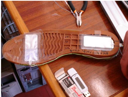
Fig. 3: First prototype of the energy generator: two piezoelectric polymer films above the sole.
