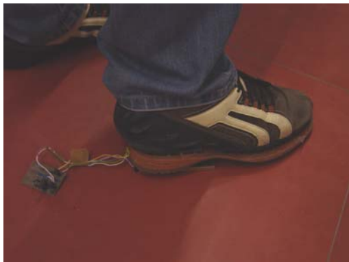
Fig. 7. Sole and electronic circuit placed in the shoe
