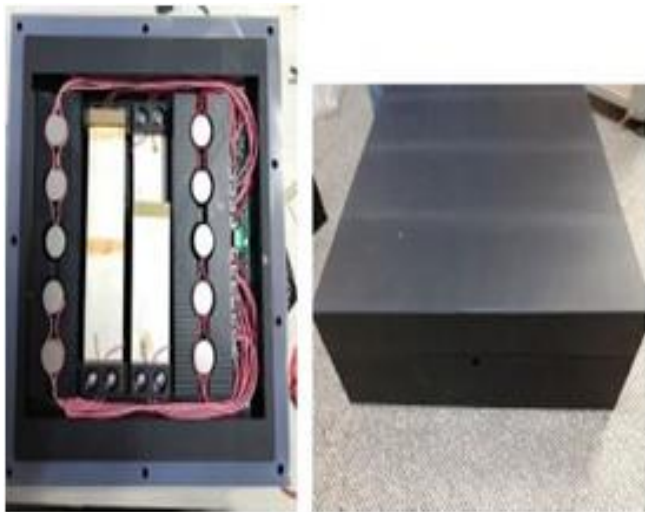
Fig 8. Piezoelectric pavement energy harvesting box (Yang et al., 2017)
