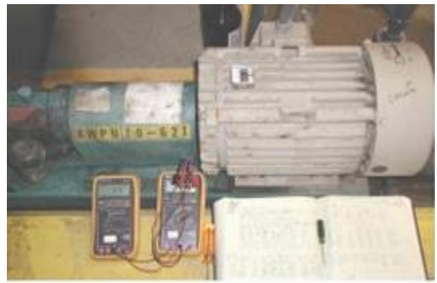
Fig 10. PEHS attached to an AC Induction motor (Khazaei et al., 2019)
