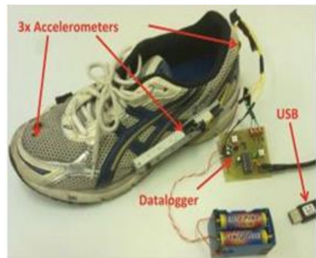
Fig 9. Shoe-sole Piezoelectric Energy Harvester (Al-Nabulsi et al., 2019)
