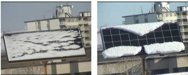
Figure 6. Snow Melting Case 1 (Patchy) and Case 2 (Slab).
