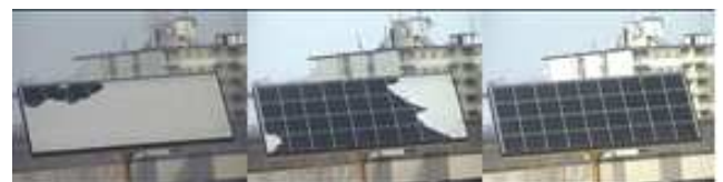
Figure 4. Complete snow melting on the panel within 20 on 4 th February from 11:55 AM to 12:05PM.
